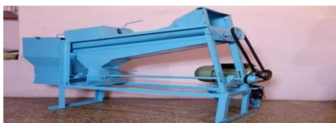
Fig. 1. Actual fabricated model of corn peeling and cutter machine.
